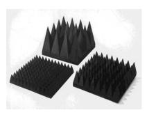
This electromagnetic absorber consists of a polyethylene foam base and utilizes the ohmic loss of carbon. Not only is the IS electromagnetic absorber capable of absorbing microwaves, it also delivers excellent electromagnetic absorption performance from as low as 300 MHz (depending on the size) through millimeter and submillimeter waves (through 1 THz).
